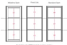
Illustration of a 1372mm high awning window. Windows 1800mm high or above come with 3 horizontal bars as standard
